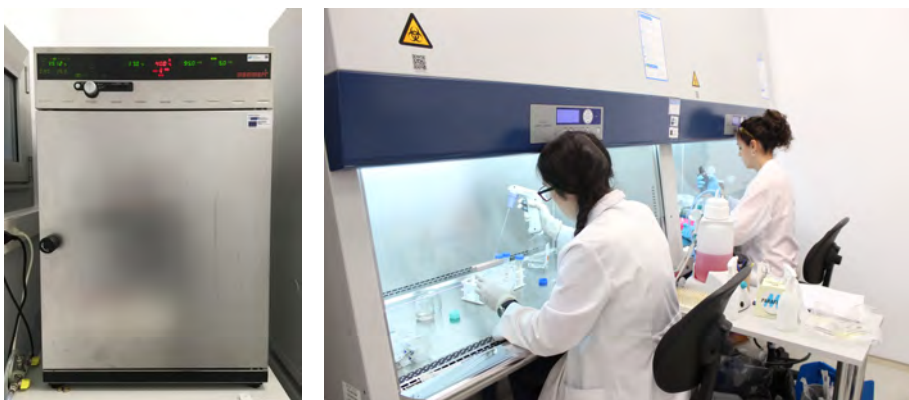
Cell culture lab equipped with a cell culture incubator (left) and two cell culture biosafety cabinets (right)
