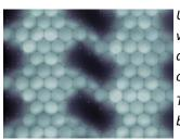
Uniformly arranged nanopores within a graphene monolayer: atomic precision and full control over its functionalisation.
